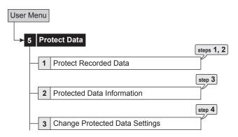
step1. Set the start and end points of the data to be locked.
